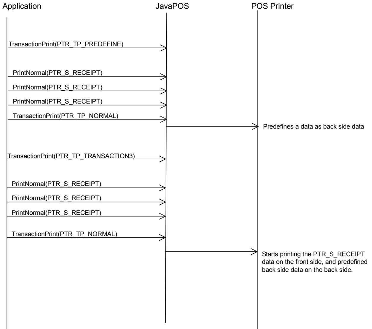
2) Example of TransactionPrint/RotatePrint for Dual Side Print
