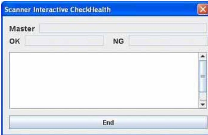
Read the bar code. The bar code read first time will be used as master data of the bar code. For subsequent bar code reading, it is judged OK if the bar code read is the same as that registered as master data. And, it is judged NG, if the bar code read is different from the master data.
