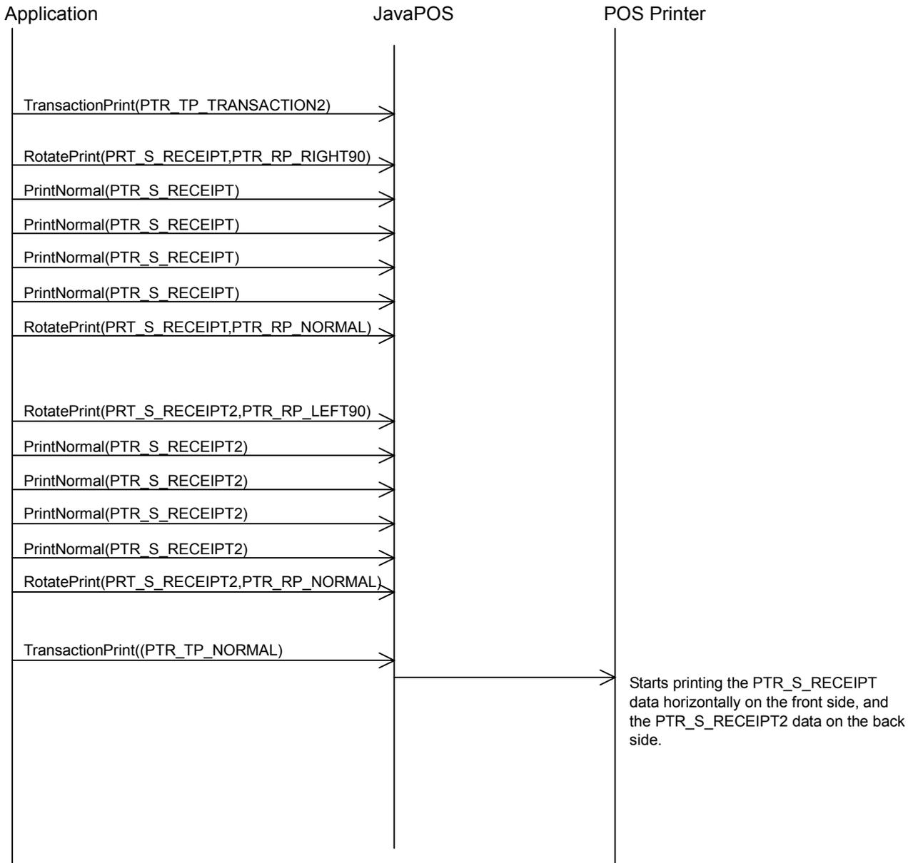
3) Example of Dual Side Print if JavaPOS registry 2STPrintingMode=1 or when TPTR\_2STCMD\_SET\_PRINTINGMODE=1 is specified by DirectIO
