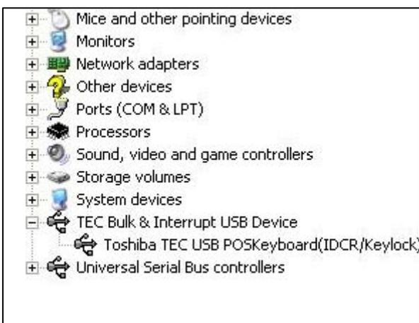
Start the Device Manager and check that the Keyboard Filter driver has been successfully installed. Then, open the system32 folder (C:¥WINDOWS¥system32) and make sure that TECPKBFilter.JNI.dll has been copied.
