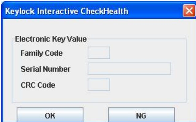
When the above window appears, make the iButton touch to the button contacts.
