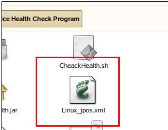
Change the name of the Linux\_jpos.xml file in the Device Health Check Program folder to jpos.xml.
