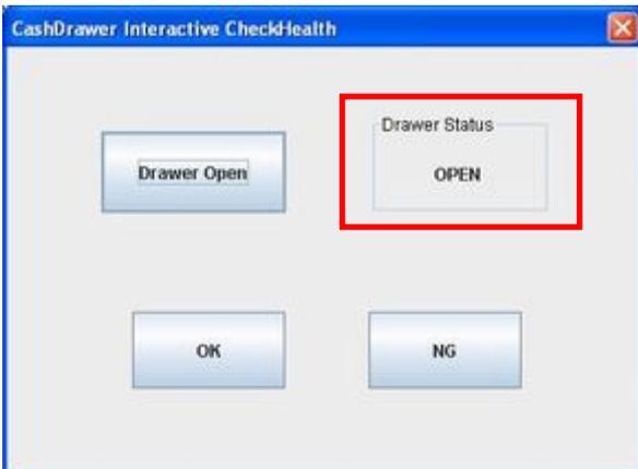
The drawer opens and a message, "OPEN" is displayed on the [Drawer Status] box at the upper right in the window on the screen.
