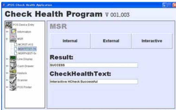
Values displayed in the [Result:] and [CheckHealth] Text boxes differ depending on the reading result. There are the following two value combinations.
