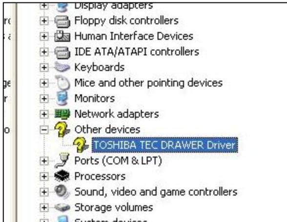
Start the Device Manager and check that the CashDrawer driver has been successfully installed. Then, open the system32 folder (C:\WINDOWS\system32) and make sure that TECCashDrawerJni.dll has been copied.
