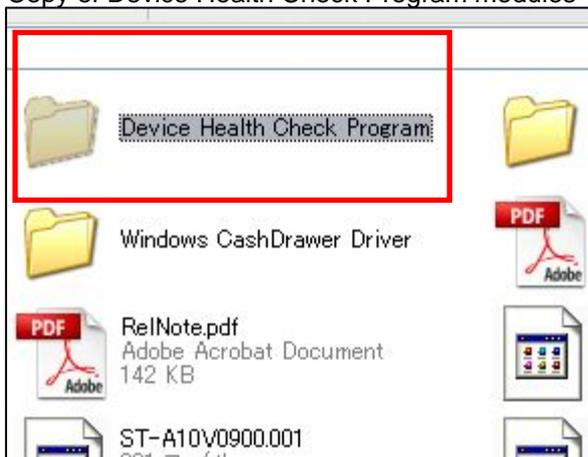
Open the Kit CD, then copy the Device Health Check Program folder to a desired location in the local computer.
