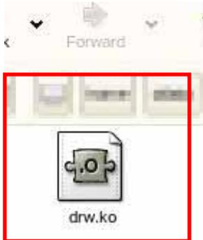
Select “Driver” → “CashDrawer Driver” → “Linux” → “Driver” → “SLED10SP1” or “SLED11”. (Please select OS used.) Copy the drw.ko driver module to any desired location.
